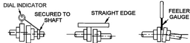
Figure 5 – Coupling Alignment
