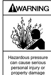
Failure to relieve system pressure prior to performing pump service can cause serious personal injury or property damage. Systems with meters will still be pressurized even after the hose is emptied
