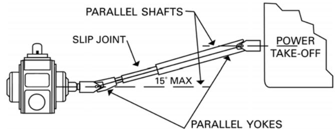
**Note: A Drive Shaft Guard between the pump and the PTO MUST be provided. (Not Shown)**
