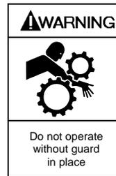
A drive shaft guard between the PTO and pump must be provided to prevent personal injury, property damage, or death.
