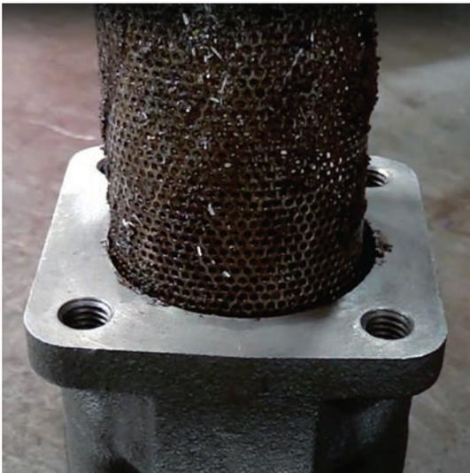
Clogged strainers signal suspended solids, which are a legitimate threat to most process pumps – and maintenance budgets.
