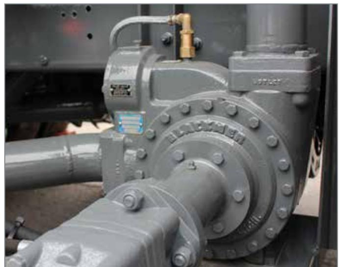
Only pumps that can reliably offer specific, steady, non-pulsing flow rates should be used on LPG delivery systems. For Robine Trucks, LGL Series Sliding Vane Pumps from Blackmer® meet these requirements.
