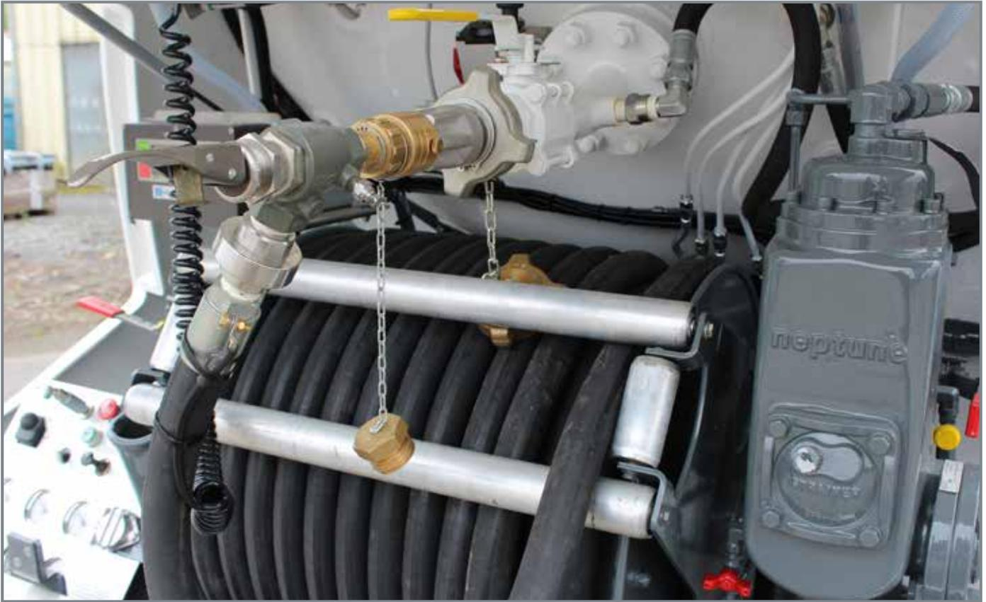
While the metering system for many years for LPG-delivery vehicles was the positive displacement, recently, LPG-transport builders have moved to a newer technology – the mass flowmeter – to measure delivery volumes.
