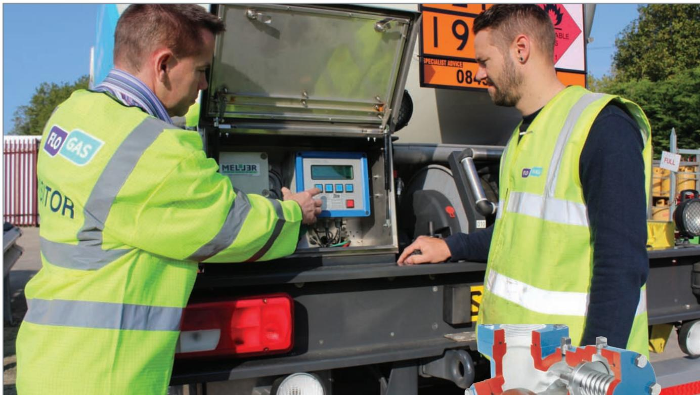
Thanks to the efforts of innovative product-transfer solution providers like UK-based Meller Flow Trans Ltd., LPG-delivery company Flogas has found a next-generation solution to keeping its LPG-delivery vehicles on the road in the form of a product-transfer and metering system that features Blackmer® LGL Series Sliding Vane Pumps and Flowcom 2000 Flow Meters.
