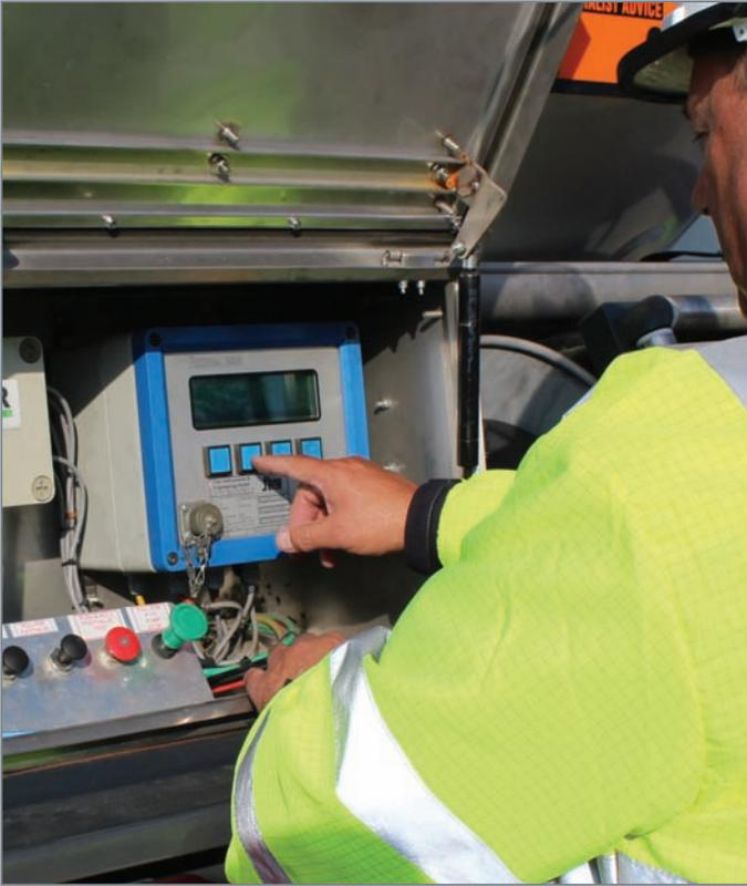
What sets the Flowcom 2000 apart from traditional meters is that it facilitates fluid transfer through venturi-based pressure-differential metering principles, rather than mechanical moving parts.
