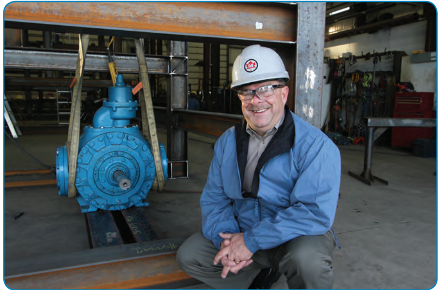
Tony Giasson next to one of the Blackmer HXL Series pumps ready to be installed on a new CO 2 transfer skid.
