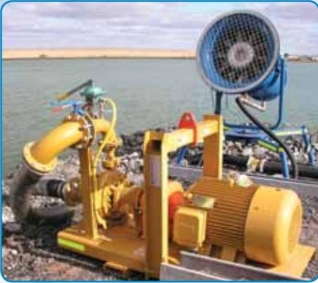
The heart of this water evaporation system in Australia is the Blackmer System One® centrifugal pump.
