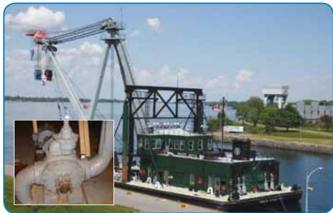
The same Blackmer GL6 Model Sliding Vane Pump has been used to pump bilge water on a barge in the St. Lawrence Seaway for more than 50 years.
