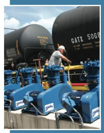
To ensure the best type of reciprocating piston compressor is selected, suppliers will ask their customers to complete a Data Sheet that details the specific operational conditions (photo courtesy of Blackmer).
