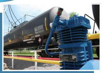
The venerable oil-free reciprocating piston compressor is often the best choice for the transfer of a wide range of industrial gases, from ammonia to vinyl chloride, thanks to a design (left) that protects the commodity being handled while controlling leakage. However, like any technology, proper consideration must be given to the demands of the product-transfer application and operational parameters before an educated decision can be made (photo courtesy of Blackmer).
