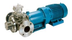
Seal-less Sliding Vane Pumps feature a magnetic coupling consisting of samarium-cobalt magnets and a unique bearing and head design that allows a small quantity of pumpage to circulate through the containment can, which minimizes temperature rise and maximizes bearing life.
