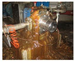
The most obvious shortcomings of mechanically sealed pumps in chemical processing are the catastrophic failures that can occur when the seals fail. In these instances, valuable raw materials and end products are irretrievably lost, while the safety of plant personnel and the environment is put at risk.
