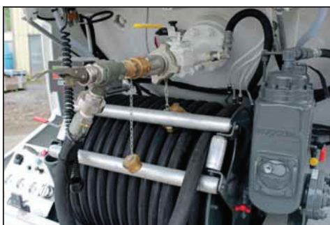
While the metering system for many years for LPG-delivery vehicles was the positive displacement, recently, LPG transport builders have moved to the mass flowmeter to measure delivery volumes.
