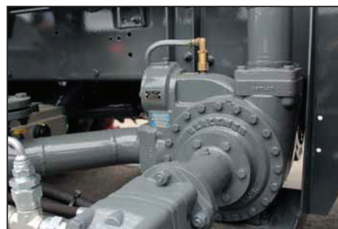
Only pumps that can reliably offer specific, steady, non-pulsing flow rates should be used on LPG delivery systems. For Robine Trucks, Blackmer's LGL sliding vane pumps meet these requirements
