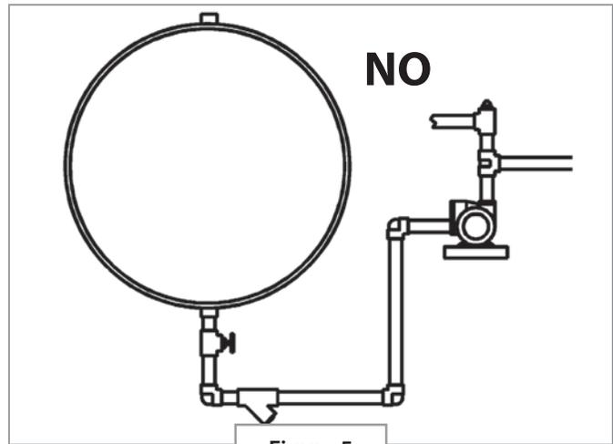
2. The pump should always be at a lower level than the tank's lowest liquid level. Install the pump to eliminate any low spots or loops in piping. **Figure 5**
