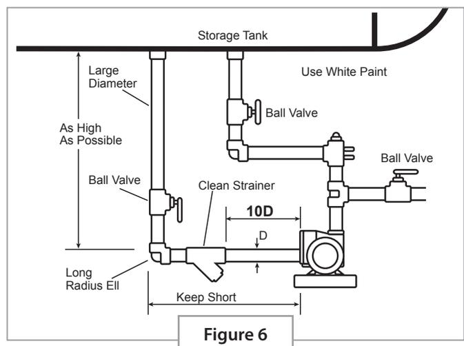
5. The nearest fitting or strainer should be a minimum of 10 pipe diameters from the pump inlet. Where possible, limit elbow connections to a maximum of 3 elbows. Use full port ¼ turn valves for component isolation. It is a good practice to install 3 full port ball valves, isolating the pump, bypass,
