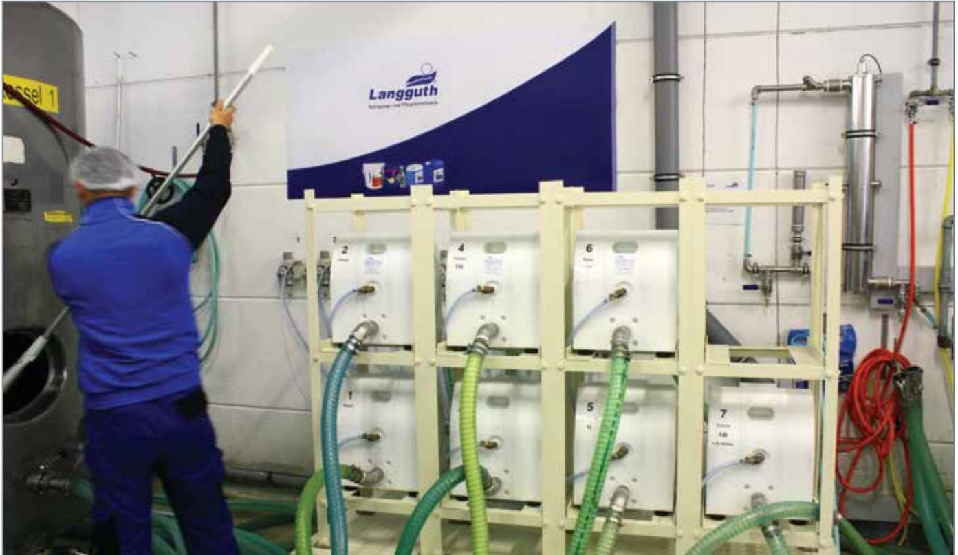
After watching a number of plastic AODD pumps fail in its continuous-duty container-filling operations, Langguth Chemie GmbH has found the perfect solution in the E40 Series Air-Operated Double-Diaphragm (AODD) Pump from Almatec.®
