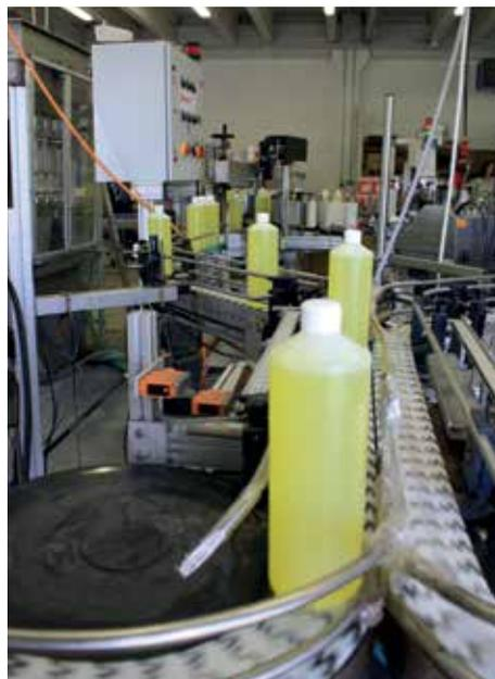
From the time a technician doses the ingredients into a mixing vessel until the end-product is bottled and sent down the packaging line, Langguth Chemie relies on AODD pumps to ensure that its manufacturing process is efficient, cost-effective, and less noisy
