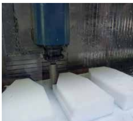
Almatec AODD pumps in a CNC machine during manufacture
