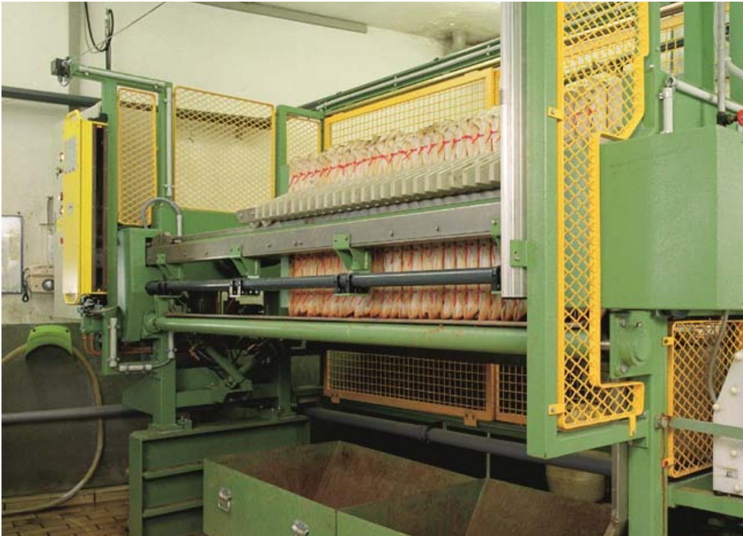
AODD pumps are a popular choice in filter-press systems because they offer reliable high-pressure operation and product containment, while being safe and easy to maintain. They are also capable of handling a wide range of slurries and chemicals that are a staple of the process.
