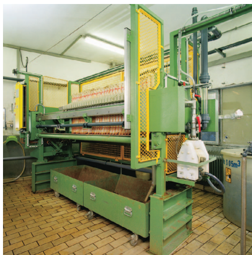
Figure 1: A typical chamber filter press being fed by a high-pressure air-operated double-diaphragm (AODD) pump (Almatec® AHD Series)
