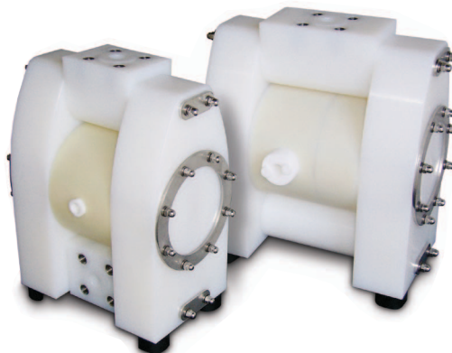
Figure 4: Almatec® offers two models of high-pressure AODD pumps for use in chamber filter presses, the AHD Series with internal pressure conversion, and the AHS Series for use with an external booster
