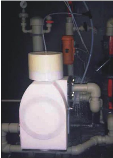
*Almatec's E-Series Plastic AODD pumps are machined from solid plastic blocks of polyethylene (PE) or polytetrafluoroethylene (PTFE), allowing the pumps to handle the harshest environments.*
