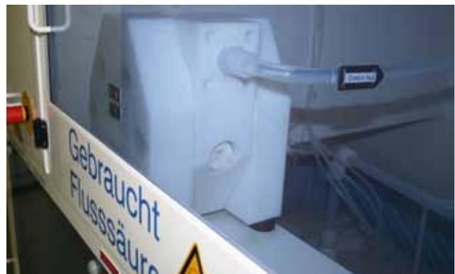
The Almatec E-Series solid-body air-operated double-diaphragm (AODD) pumps represent one of the safest, most durable and effective option for transferring hazardous chemicals.
