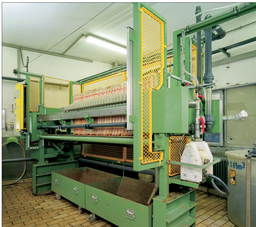
Figure 1: Chamber filter press with an Almatec air-operated double-diaphragm pump
