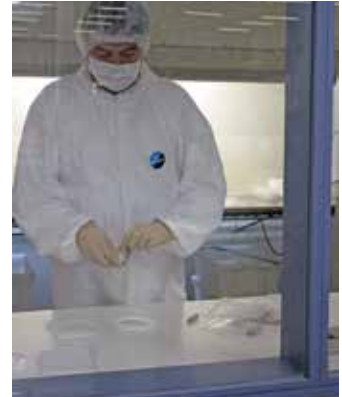
A clean room is used to hygienically prepare all the pumps and equipment for clean-room applications.
