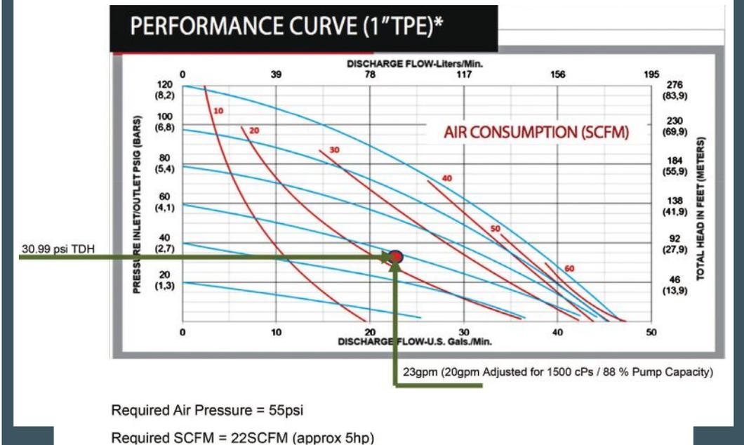
Viscosity and pipe diameter play a significant role in suction line loss and must be considered during evaluation. The system capabilities are limited by the pump's suction lift capabilities and air-inlet pressure. ■
