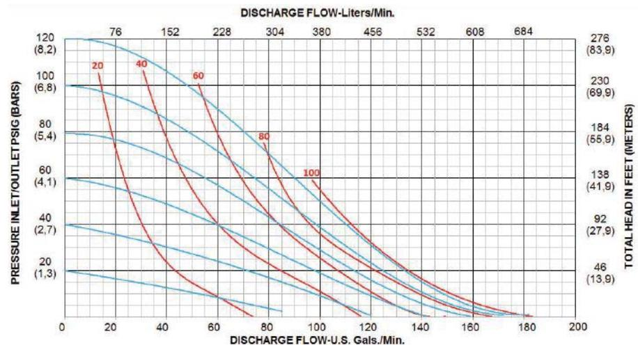
Figure 8a: Performance curve measured using PTFE diaphragm.
