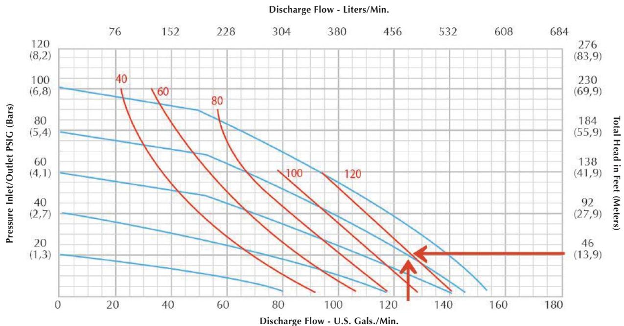
Figure 1: All-Flo's Legacy Product Performance Curve, an illustration of a performance curve for a typical 2-inch (50.8 millimeter) AODDP.
