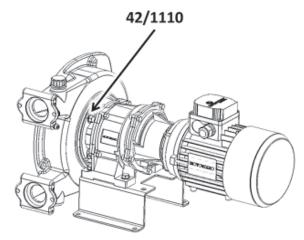
Refit rotor in the pump (see § ROTOR REMOVAL), refit hose (see § HOSE REPLACEMENT) and fill the pump with lubricant (see § LUBRICANT REPLACEMENT).
