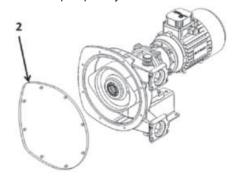
Screw and tighten screws 33 and their washers 34, starting by top ones to secure cover assembly. Tightening torque 1 + 0,2 N.m.
