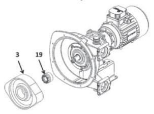
Position rotor 3 to have distance B between rotor outer edge and casing 1 back wall.
