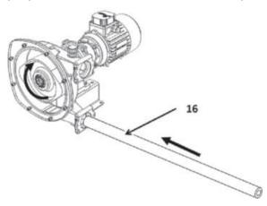
If pump rotates anti-clockwise, suction is on the top port :
