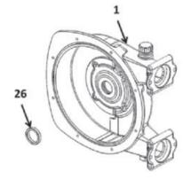
Make sure the shaft seal is in the right direction :
