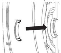
If necessary to replace friction ring 27, use a mallet and a chisel, to break and remove friction ring 27.
