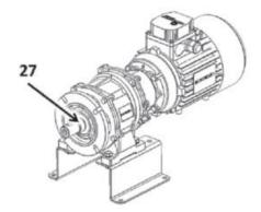
Let friction ring cool down before carrying on reassembly. Put back the pump body.
