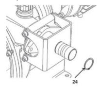
4. Fit screws 1106 with their washers and tighten them. **Tightening torque 15 ± 2 N.m**.
