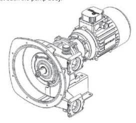
Put back nuts 42 and their washers 1110 and tighten them. **Tightening torque 19 N.m**.
