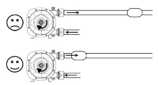
Change pumping set or pump ports position rather than multiplying pipe bends.
