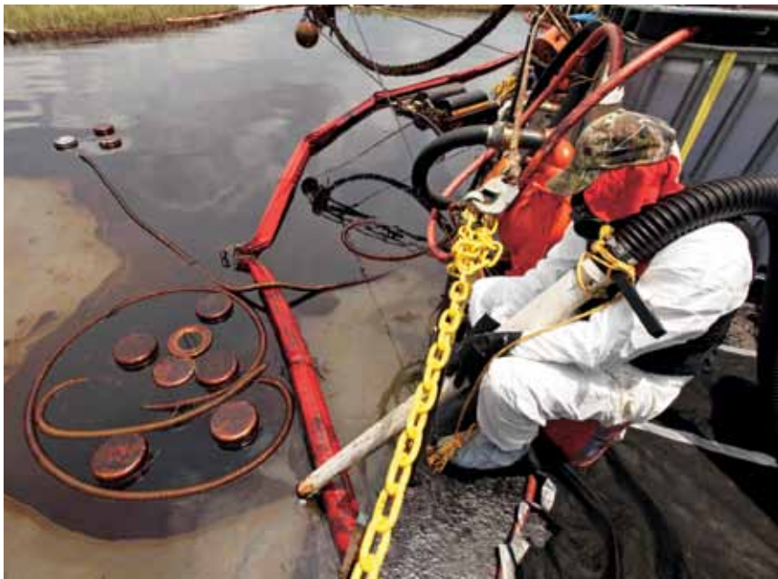
A worker cleans up oil from the Deepwater Horizon oil spill along the Northern shores of Barataria Bay in Plaquemines Parish, La., using a Wilden AODD pump.
