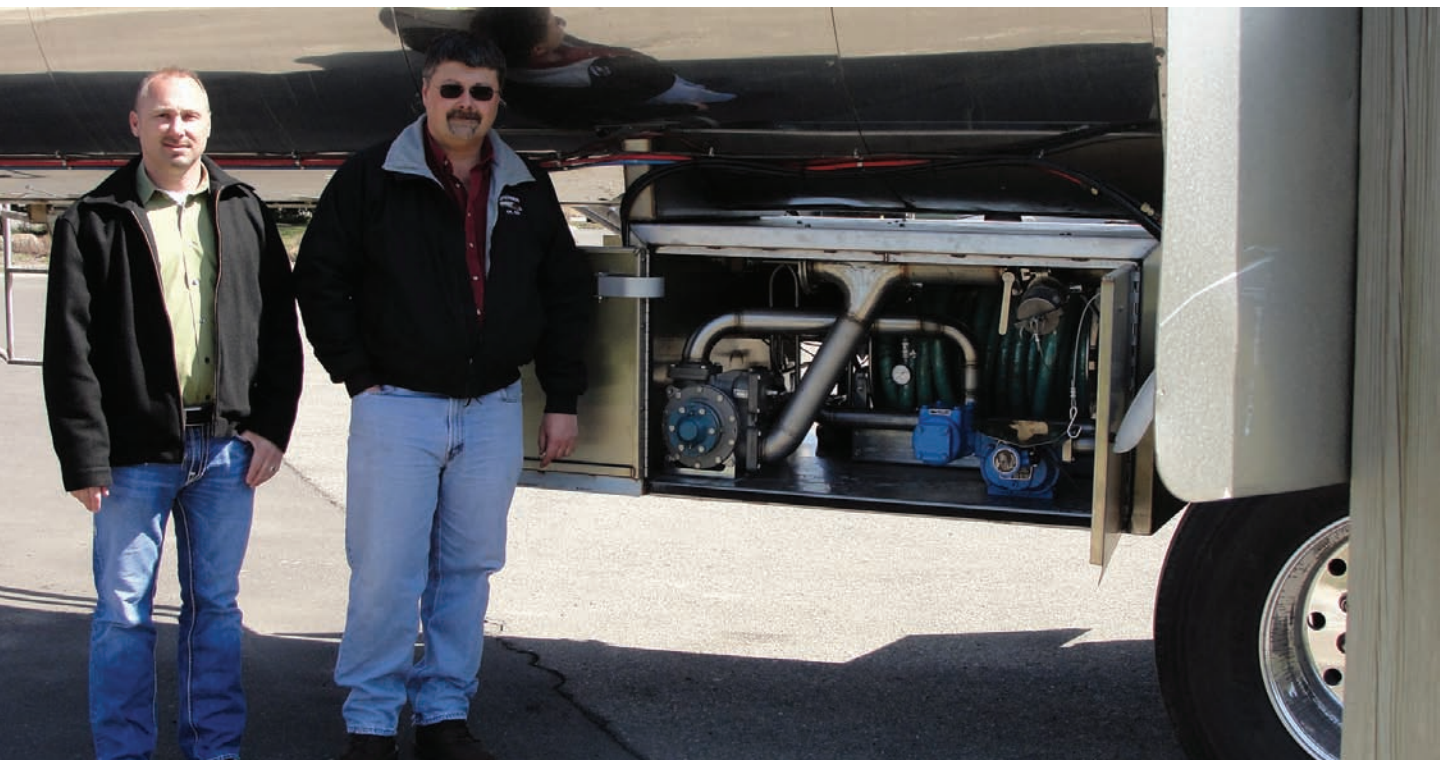
Doug (left) and Jerry Brenner, owners of Brenner Oil, Holland, MI, stand next to the company's new diesel exhaust fluid (DEF) transport. The first-of-its-kind DEF trailer was built by Liquid Haulers Maintenance, Moline, MI, and features a Blackmer® STX3-DEF sliding vane pump.
